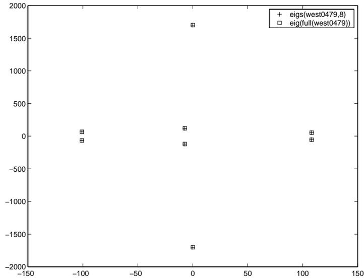
**Example 3:**  $A = \text{delsq}(\text{numgrid}('C', 30))$  is a symmetric positive definite matrix of size 632 with eigenvalues reasonably well-distributed in the interval (0 8), but with 18 eigenvalues repeated at 4. The `eig` function computes all 632 eigenvalues. It computes and plots the six largest and smallest magnitude eigenvalues of  $A$  successfully with:
