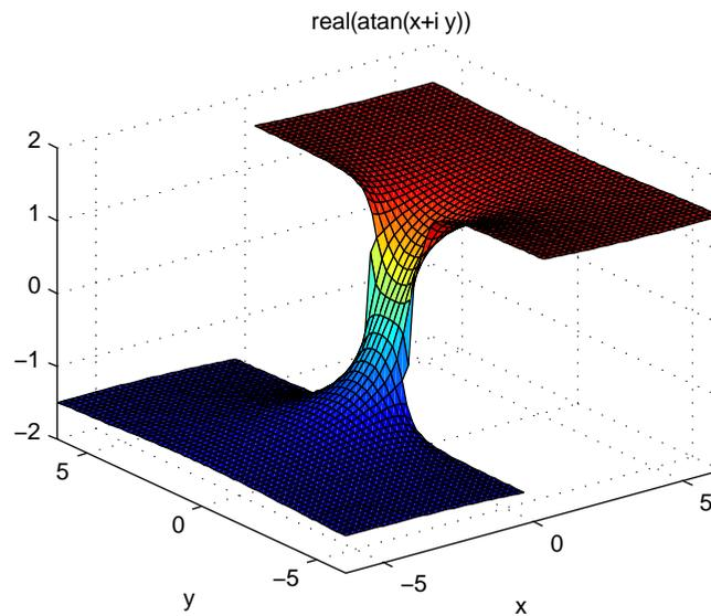
Using `surf` to plot the same data produces a graph without filtering of discontinuities (as well as requiring more steps):
