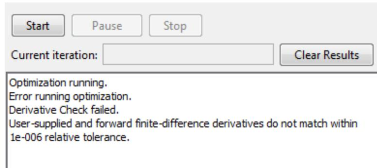
The forward finite difference approximation is inaccurate enough near  $[0 \ 0]$  that the derivative check fails.
