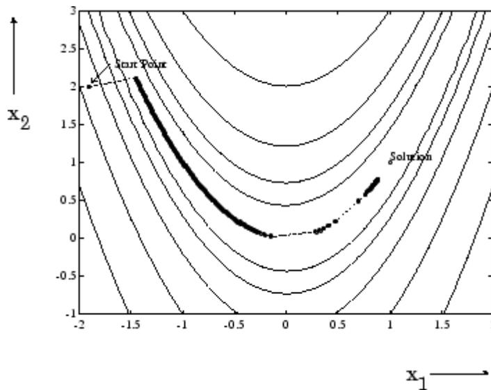
**Figure 6-1: Steepest Descent Method on Rosenbrock's Function (Equation 6-6)**
