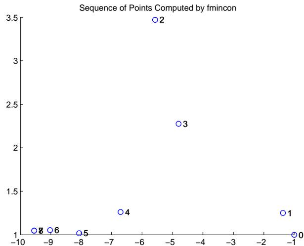
The optimal point occurs at the eighth iteration. Note that the last two points in the sequence are so close that they overlap.
