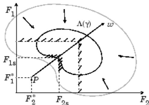
**Figure 6-5: Geometrical Representation of the Goal Attainment Method**
