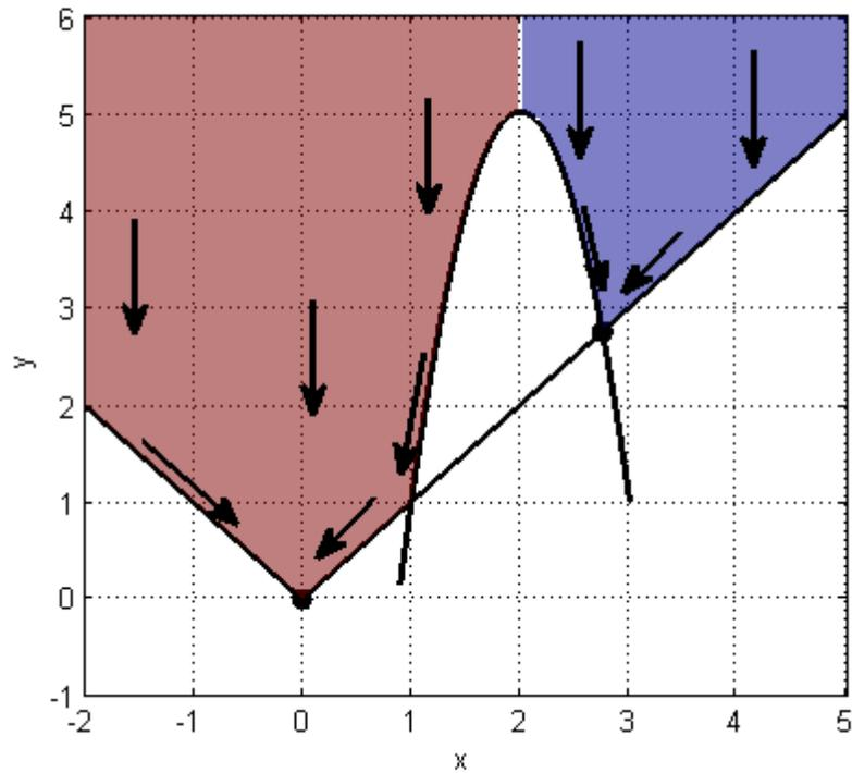
The steepest descent paths are straight lines down to the constraint boundaries. From the constraint boundaries, the steepest descent paths travel down along the boundaries. The final point is either  $(0,0)$  or  $(11/4,11/4)$ , depending on whether the initial  $x$ -value is above or below 2.
